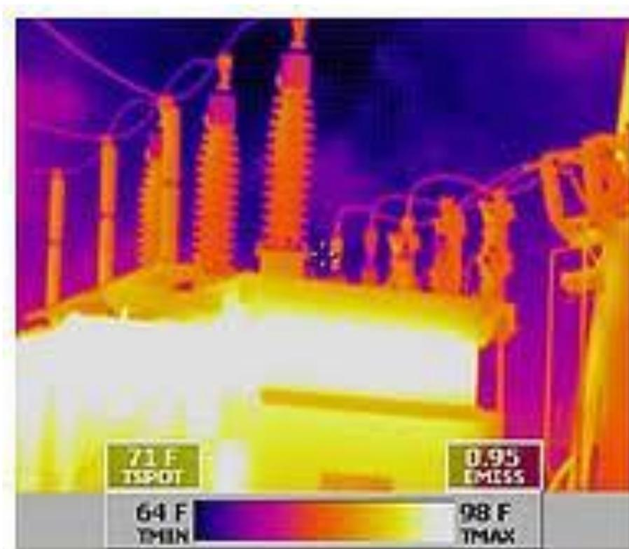
Load = Heat This Transformer Is Hot Because It Is Loaded Up
